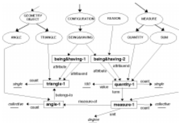
Figure 4: Semantic structure built by the NLU component for the input sentence: "It's a triangle, so the sum of its angles is 180" Ovals denote concepts, rectangles denote individuals, and underlined text denotes a constant.
